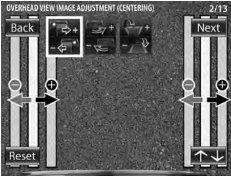
Adjustment is possible by one step to the left and right. If the adjustment is not possible in the currently available range, change the camera position before retry.
