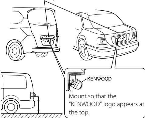
The CMOS-300 should be installed at a height of 55 cm (21.7 inch) or more.
