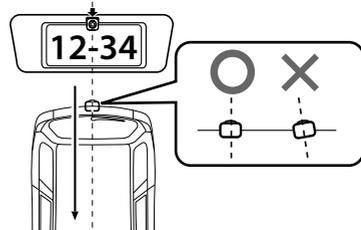
Attach the camera on the rear center position of the vehicle taking care not to hide the license plate. Make sure that the camera points straight toward the rear of the vehicle travel direction. Be careful not to lean the camera toward other directions of the vehicle, etc.
