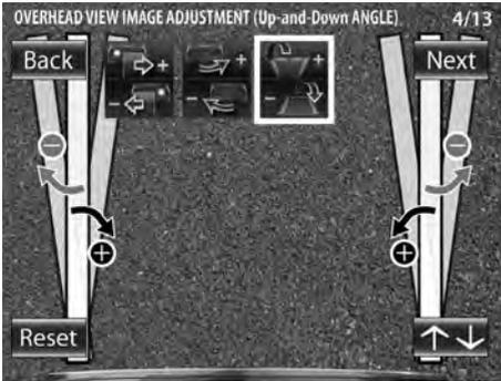
Adjustment is possible by one step up and down. If the adjustment is not possible in the currently available range, change the camera position before retrying.
