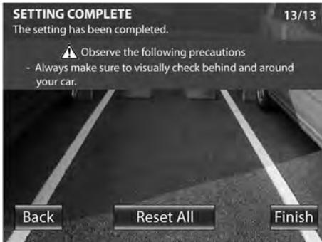
**1** Press the + or – button of the switch unit to select [Finish] and press the view button.
