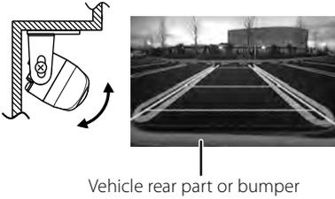
When adjusting the camera angle, be careful not to stretch the camera cord.
