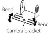
Adjust the camera bracket shape so that it fits the camera installation position.
